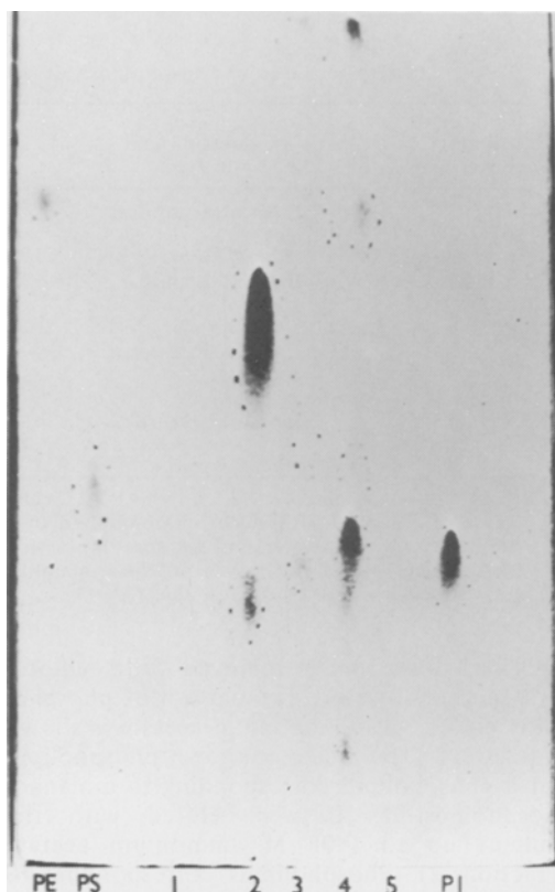
FIG. 2. Thin layer chromatogram of the Corynebacterium diphtheriae phospholipid fractions eluted from the DEAE-cellulose column. PE, phosphatidylethanolamine; PS, phosphatidylserine; 1, early elutes from the column; 2, phospholipids eluted with 0.05 M ammonium acetate; 3, 4, 5, material eluted with higher concentrations of ammonium acetate; PI, phosphatidylinositol. Chromatography was carried out on long (40 cm) plates of Silica Gel H in chloroform-methanol-water (65:25:4). Dimannophosphoinositide C' (Table II) is not obvious on this photograph. Dotted areas contained lipids which reacted with iodine previous to visualization with the phosphate spray.
