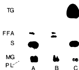
FIG. 1. A, sporophore total lipids; B, mycelial total lipids; C, triolein and cholesterol. PL, polar lipid; MG, monoglyceride; S, free sterol; FFA, free fatty acid; TG, triglyceride (The TG spot in fractions A and B formed faint spots not visible in this photograph).
