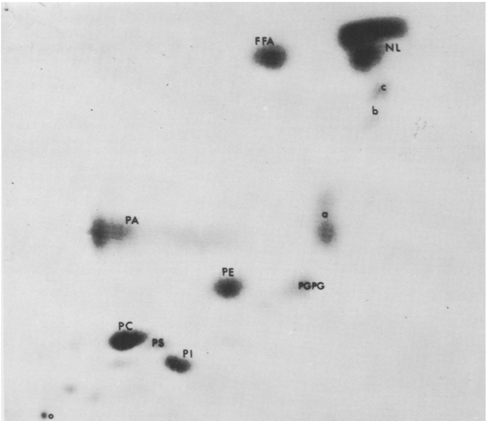
FIG. 4. Radioautogram of a thin layer chromatogram of the polar ^{14}\text{C} -labeled lipids of H. grisea var. thermoidea . The plate was developed in the x-direction with chloroform-methanol-water-28% ammonia (130:70:8:0.5 v/v) and with chloroform-acetone-acetic acid-methanol: water (100:70:20:20:10 v/v) in the y-direction.
